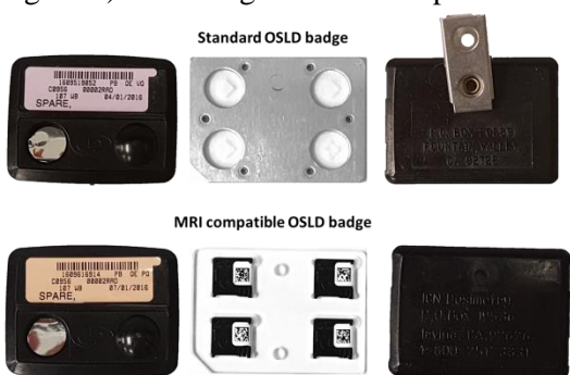
Figure 3. Design of MRI compatible OSLD badge
